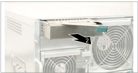
Figure 47: Removing the dummy module
